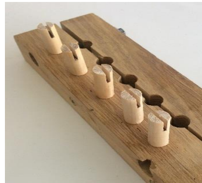
Figure 18-15. Slots Cut in Honey Bee Hubs
