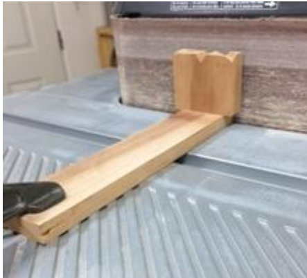
Figure 20-4. Jig Clamped to Table
