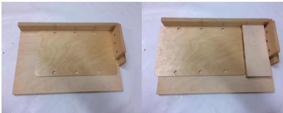
Figure 19-16. Drilling the Doll Bed Base
