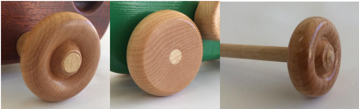
Figure 22-1. Squared off and Chamfered Axles
