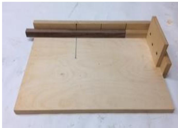
Figure 19-15. Drilling Center Hole in Rail
