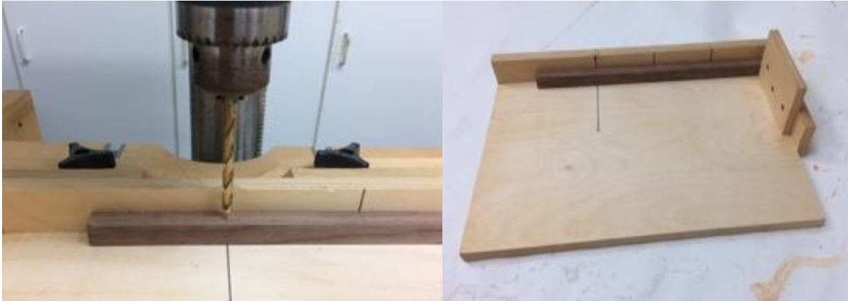
Figure 19-14. Drilling Three Holes for the Bed Rail Spacers
