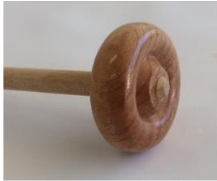
Figure 20-2. Chamfered Dowel to Form a Hub Cap
