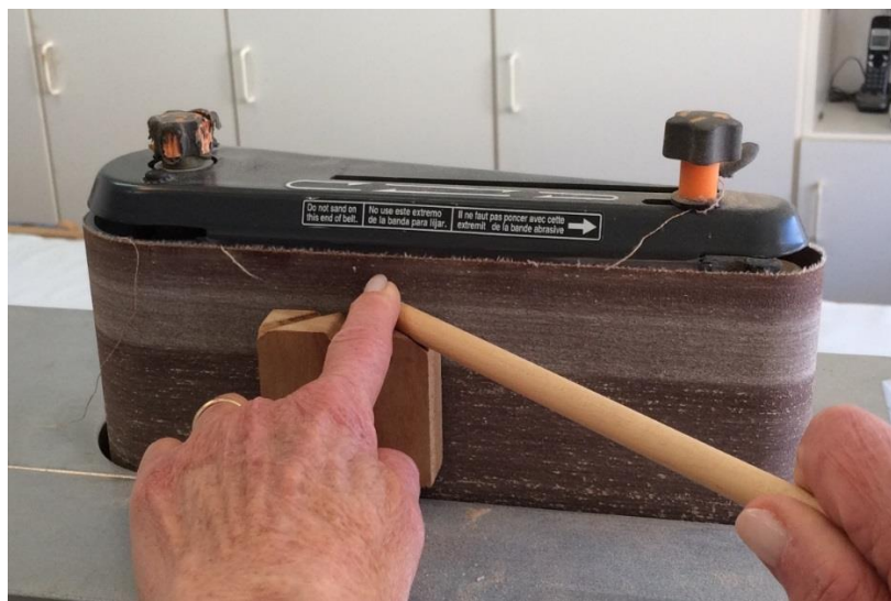
Figure 20-5. Chamfering the End of a Dowel
