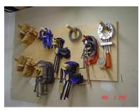
The clamps I use most often are trigger-action mini bar clamps. They're lightweight, adjust quickly and best of all, can be used with just one hand. Just slide em in position, squeeze until tight, and move on. This allows
